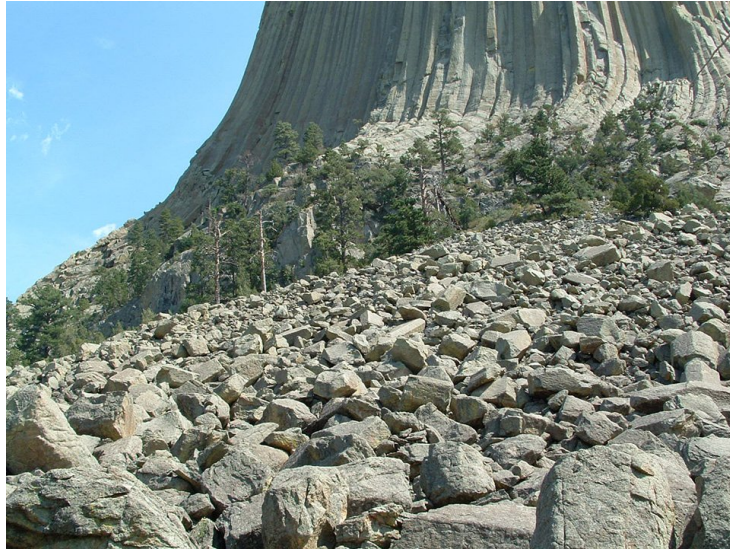
Photo P04. Rockfall blocks at the base of Devils Tower. Map the source, travel path, and deposition area separately. An old talus deposit establishes past activity but does not by itself establish current rockfall frequency. NPS. Source ; Public domain (NPS credit) .
