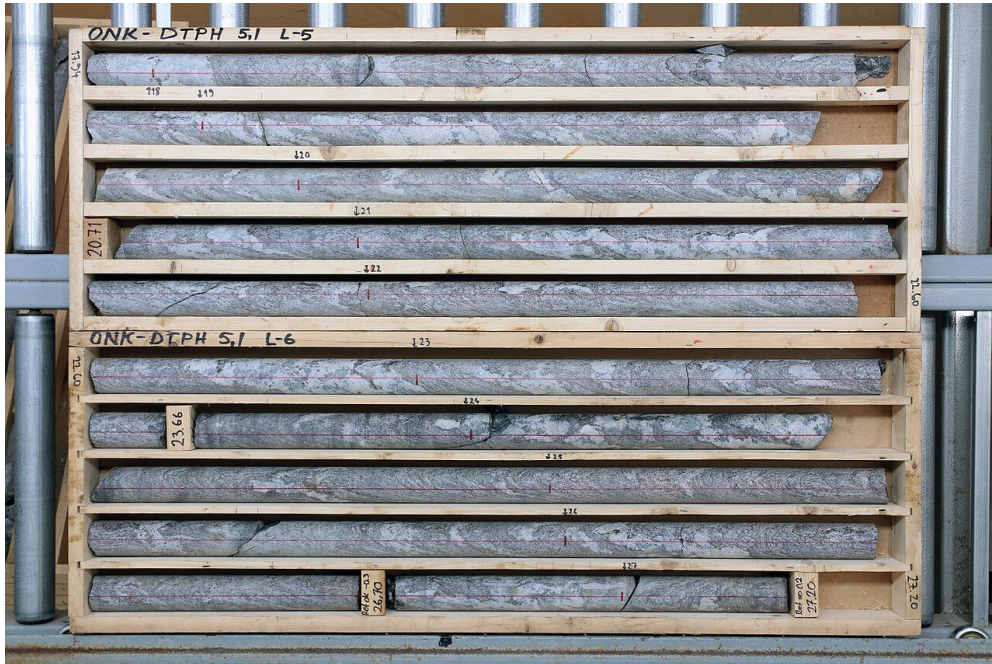
Photo P15. Ordered core boxes from Onkalo, Finland illustrate why run markers and original core order matter. RQD requires run length, soundness, and natural-versus-drilling-break judgment; do not calculate RQD from this overview photo. kallerna. Source ; CC BY-SA 4.0.
