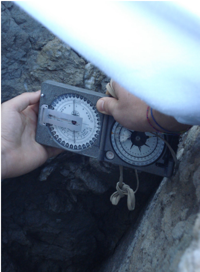
Photo P12. The compass is held horizontally to measure a geographic bearing associated with the inclined surface. Write down whether your bearing is strike or dip direction and which north reference you used. Meanos. Source; Public domain (photographer dedication) .
