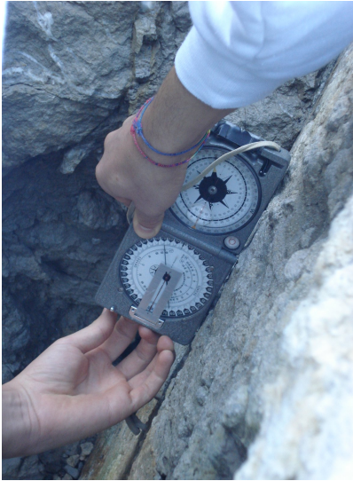
Photo P11. A clinometer is held vertically against a fault surface to measure inclination. Seek the maximum downward inclination for true dip; measure the bearing separately with the compass horizontal. Meanos. Source; Public domain (photographer dedication) .
